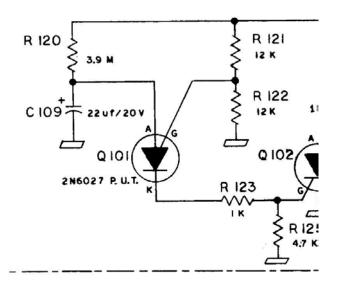
The only other "weak" point I find in the circuit, is the reed relay K6. Either C109 & K6 replacement should cost less than \$3 each.
